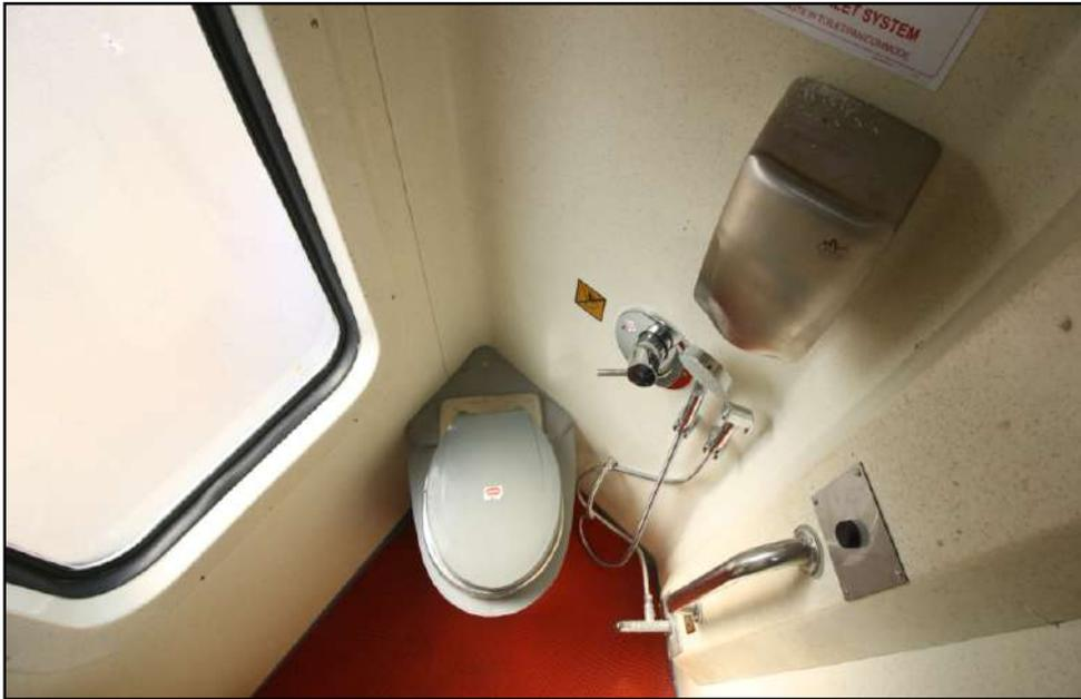
Shower Cubicles with Hot & Cold Running Water is available on board. Lavatories are equipped with Bio Toilets with Vacuum evacuation.
